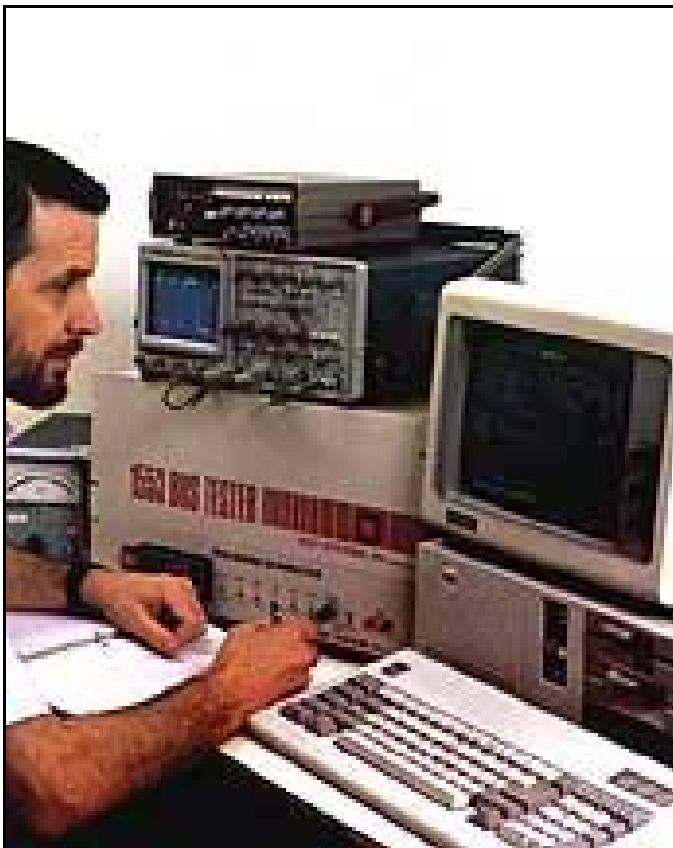
Test set-up for MIL-Std-1553 remote terminal validation testing.
