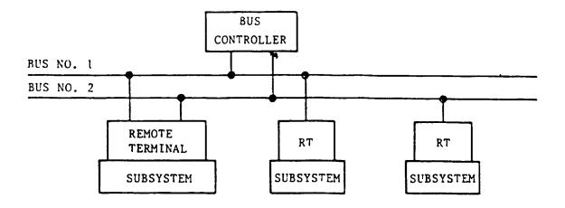
FIGURE 11. Illustration of possible redundancy.
